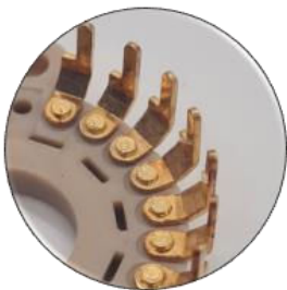
Hot riveting of contacts
