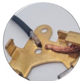
Welding of compacted cables
